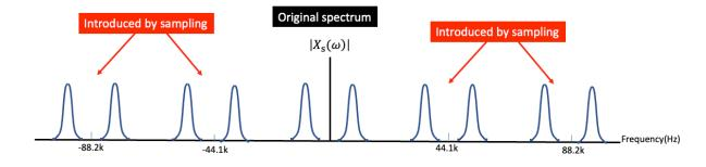
b) The 15kHz tone is clearly from the bat's echolocation, aliased to this frequency. The folding back is mirroring at ½ fs, or 22.05kHz.
