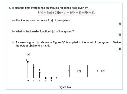
This question tests student's understanding of discrete-time systems, impulse response, transfer function in the z-domain, difference equation and the idea of convolution.
